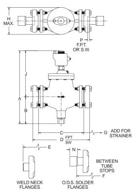
Allow 100mm (4") above valve for removal of coil housing assembly. Allow 25mm (1") below valve to operate manual opening stem.
