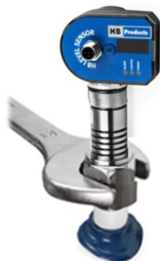
Figure 3: Mount the sensor on the vessel. Torque 80-150 Nm.
