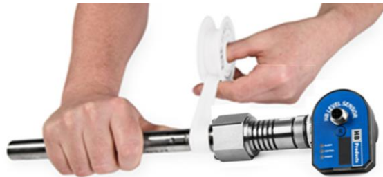
Figure 1: To install the sensor Teflon tape (NPT) or sealing washer (BSPP) is required.
