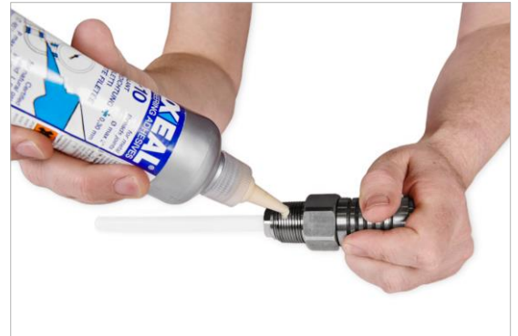
Apply liquid gasket / Teflon to the conical thread.
