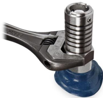
Install and mechanically tighten in the vessel, and tighten depending on the thread type and size (80-150Nm).
